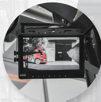
Display Screen (Featuring Power display, hour meter, and fault diagnosis)
