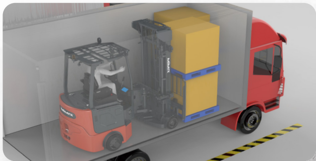
Low mast design enables handling inside containers
